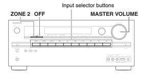
To turn on Zone 2 and select an input source, press ZONE 2 followed by an input selector button within 8 seconds.
